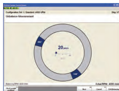
Pre-Balancing: Spread angle method
